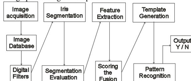
Fig. 12 : Block diagram of a typical biometric scheme for the iris recognition-I
