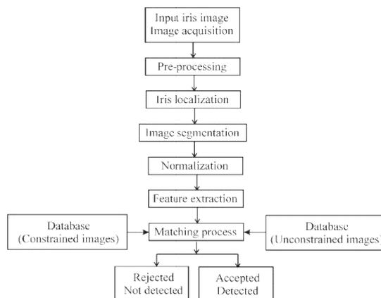
Fig. 20 : General flow-diagram of the biometric authentication process (DFD)
