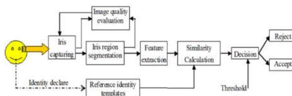
Fig. 13 : Block diagram of a typical biometric scheme for the iris recognition-II
