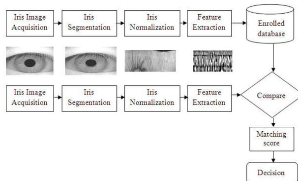
Fig. 21 : General biometric authentication process block diagram
