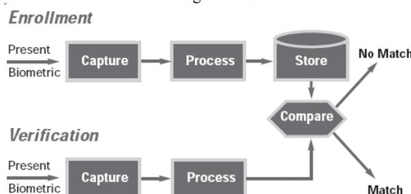
Fig. 14 : Block diagram of a typical biometric scheme for the iris recognition-III
