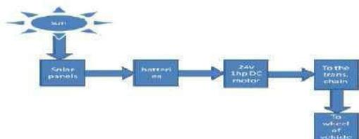
**Fig.1 Basic block Diagram Representation of Solar vehicle**
