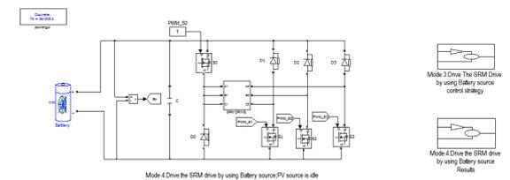
Mode 4: Drive the SRM drive by using Battery source; PV source is idle
