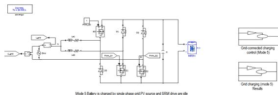
Mode 5: Battery is charged by single phase grid; PV source and SRM drive are idle
