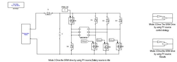
Mode 3: Drive the SRM drive by using PV source; Battery source is Idle
