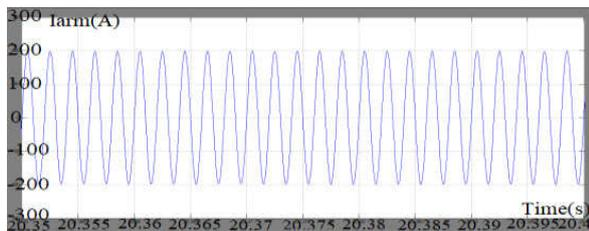
Fig.26:Arm current when the frequency is varied from 4Hz to 50Hz and 50Hz to 4Hz with Time(s) and Zoomed at transition of dc bus voltage from 100% to 50% around 20.5sec
