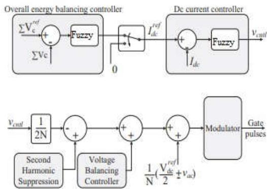
Fig.7 Block diagram of the control scheme.
