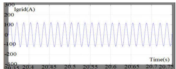
Fig.30:Grid current when the frequency is varied from 4Hz to 50Hz and 50Hz to 4Hz with Time(s) and Zoomed at transition of dc bus voltage from 100% to 50% around 20.5sec
