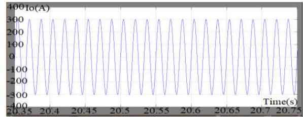
Fig.28:Output current when the frequency is varied from 4Hz to 50Hz and 50Hz to 4Hz with Time(s) and Zoomed at transition of dc bus voltage from 100% to 50% around 20.5sec
