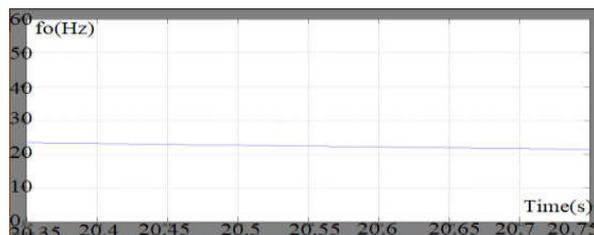
Fig.20: Output Frequency when the frequency is varied from 4Hz to 50Hz and 50Hz to 4Hz with Time(s) Zoomed at transition of dc bus voltage from 100% to 50% around 20.5s
