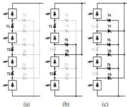
Fig.5. Different switching states of the rectifier for : a) rated dc bus voltage, b) 50% of rated dc bus voltage, c) 25% of rated dc bus voltage.
