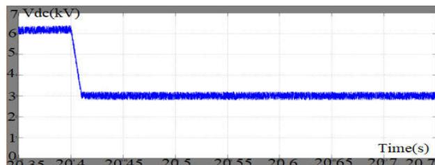
Fig.22: Dc bus voltage when the frequency is varied from 4Hz to 50Hz and 50Hz to 4Hz with Time(s) Zoomed at transition of dc bus voltage from 100% to 50% around 20.5s
