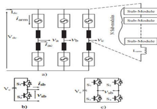
Fig.1: Circuit configuration of a modular multilevel converter. a) Three phase converter, b) half bridge submodule, c) full bridge submodule.
