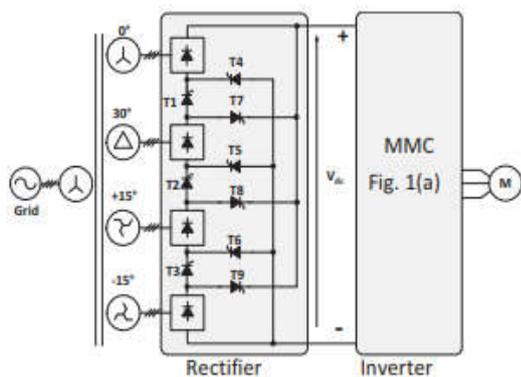
Fig.4. Proposed configuration of the MMC based drive
