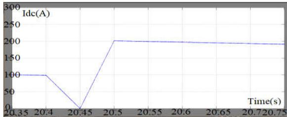
Fig.24 Dc current when the frequency is varied from 4Hz to 50Hz and 50Hz to 4Hz with Time(s) and Zoomed at transition of dc bus voltage from 100% to 50% around 20.5sec
