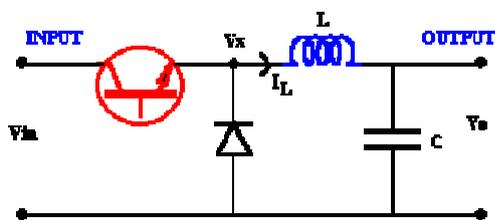
Fig.2. Buck Converter
