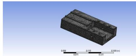
In this stage Force and displacement boundary condition were applied as follows forces, front end of the machine bed carries cutting force, weight of the work table and weight of the work piece, due to this a total load of 272 N is applied on the Guide ways of Machine bed. Rear end of the Machine bed carries vertical column, and other accessories (ie servo motors, spindles etc.), due to this a total load of 717N will be applied on two flat surfaces of rear end.
