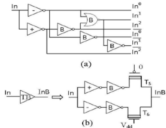
Fig: 2 Schematic diagram of (a) Ternary Decoder (b) Ternary buffer (TB)
