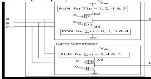
Fig: 1 Schematic diagram of Proposed CNTFET-based TFA cell
