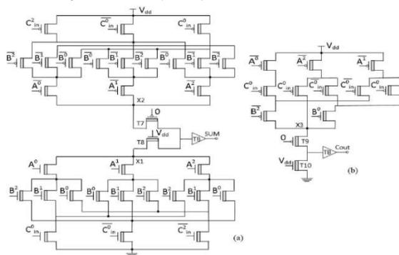
Fig: 3 Transistor level implementation of Proposed CNTFET-based TFA cell
