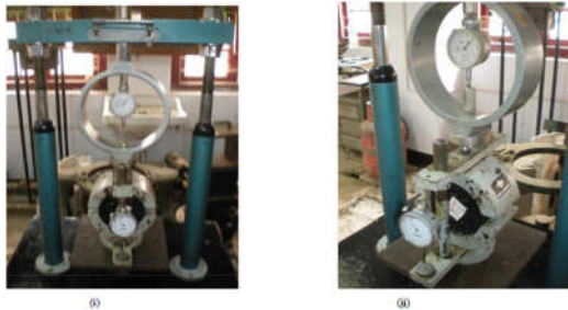
Fig. 2.1 Marshall test in progress
