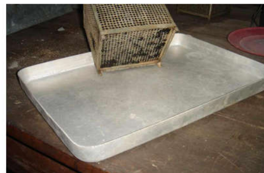
Fig. 2.6 Drainage of CRMB 60 binder sample
