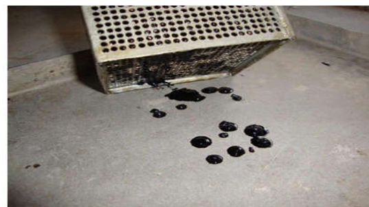
Fig. 2.5 Drainage of 60/70 bitumen sample
