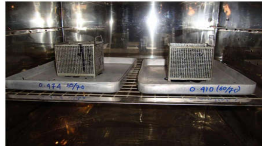
Fig. 2.3 Drainage baskets kept in oven at 150°C
