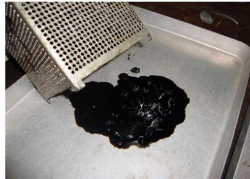
Fig. 2.4 Drainage of 80/100 bitumen sample
