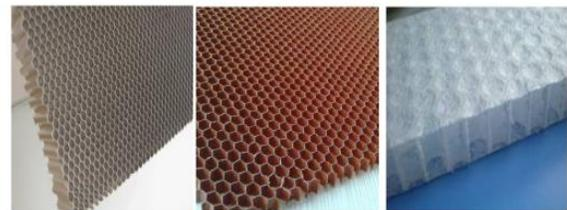
(a) Aluminum honeycomb (b) paper honeycomb (c) polypropylene honeycomb
