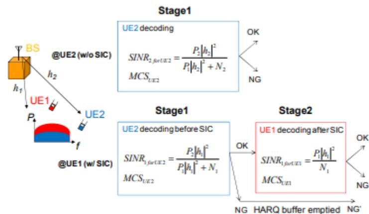
Fig. 2. Error propagation modeling.
