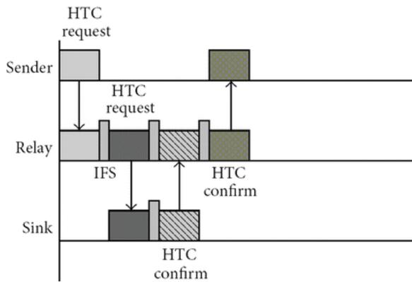
**Figure 2** Sequence chart of the establishment of HTC algorithm.
