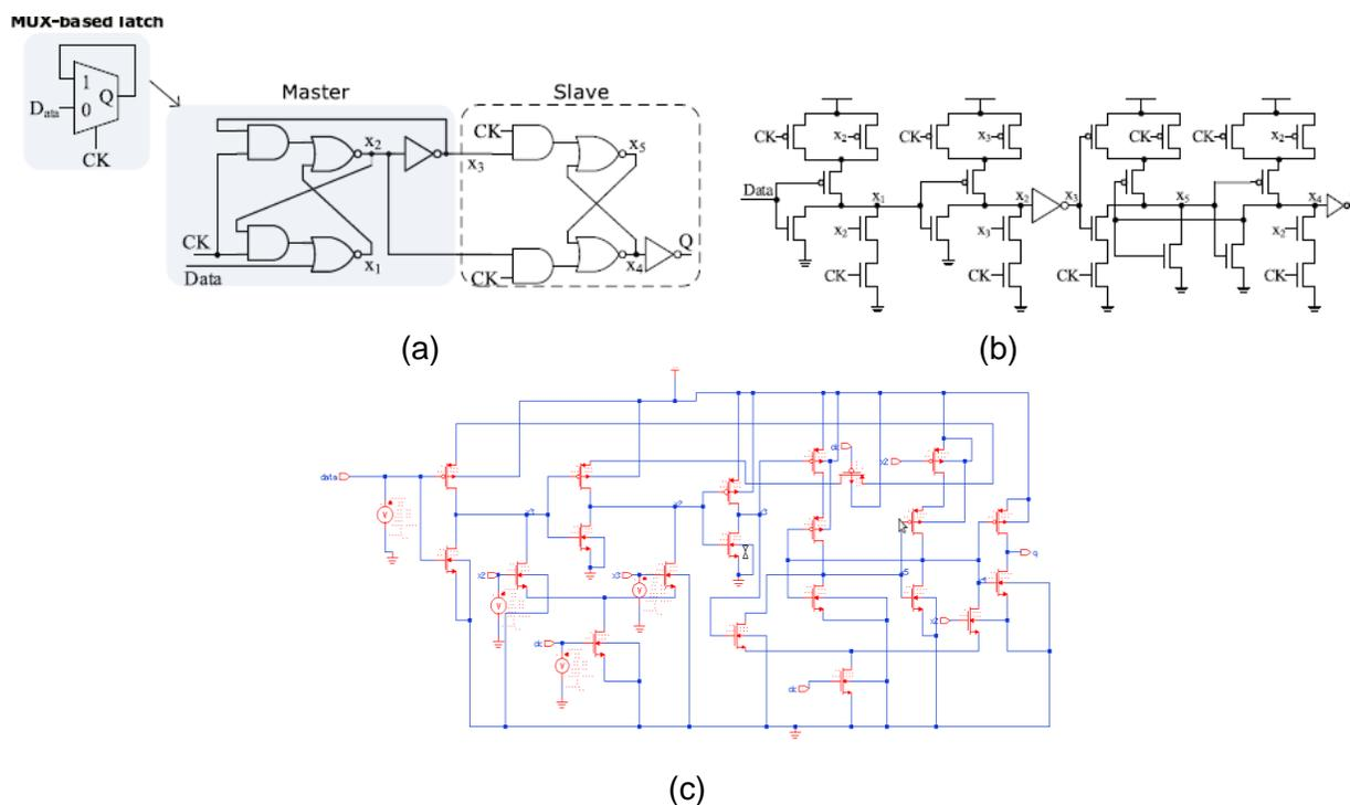
Fig. 2. TCFF. (a) logic structure. (b) MOS circuit schematic(28 transistor). (c) TCFF(21 transistor)
