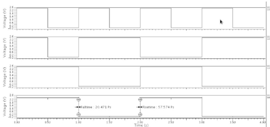
Fig.5. Simulation results for 18 Transistor Flip-Flop
