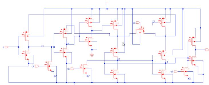
Fig. 4. Proposed circuit 18 transistor TSPC Flip-Flop design
