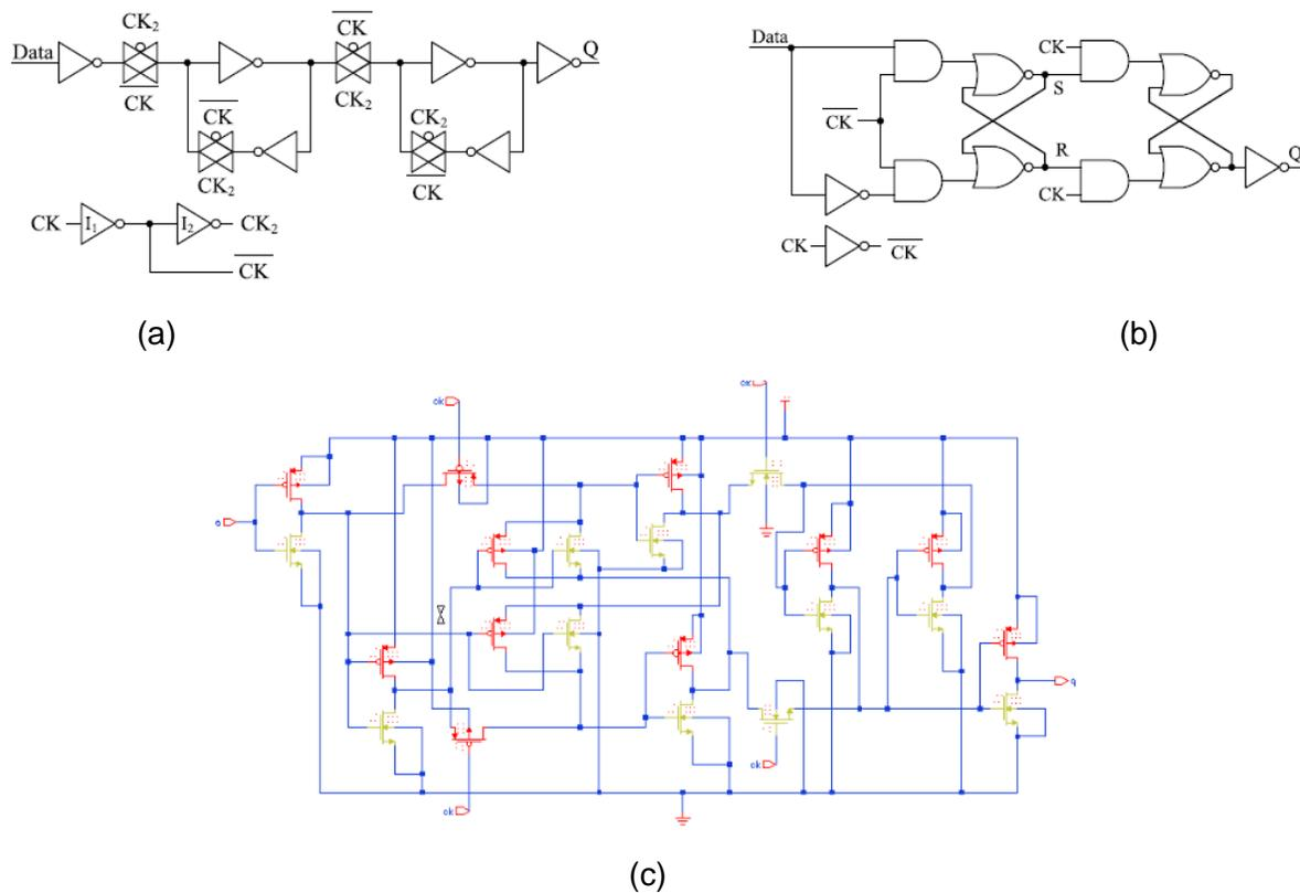
Fig. 1. Conventional fully static FF designs (a) TGFF (b) SRFF (c) ACFF
