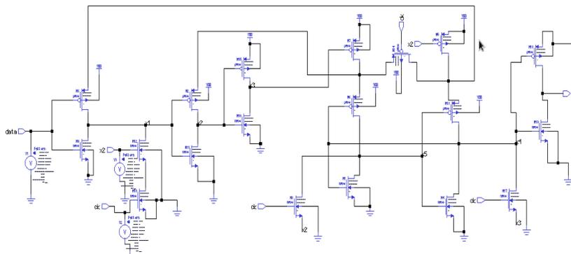
Fig. 3. LRFF(Logic Structutre Reduction Schemes Flip-flop)
