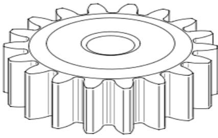
Fig 3.3 Spur Gear
