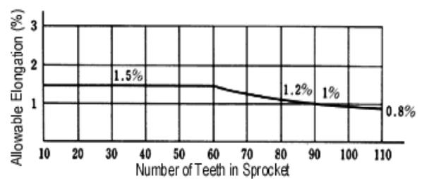
Fig 3.2 Chain's wear elongation limit
