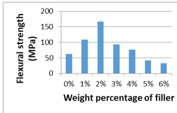
**Figure 4. Flexural strength of specimens at different filler percentages**
