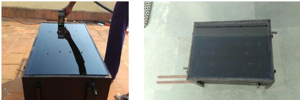
**Figure 3. Assembled view of solar air heater with glass plate**
