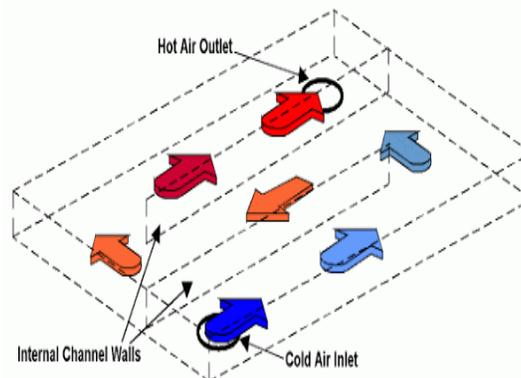
**Figure 1. Flow Diagram of Solar Air Heater**
