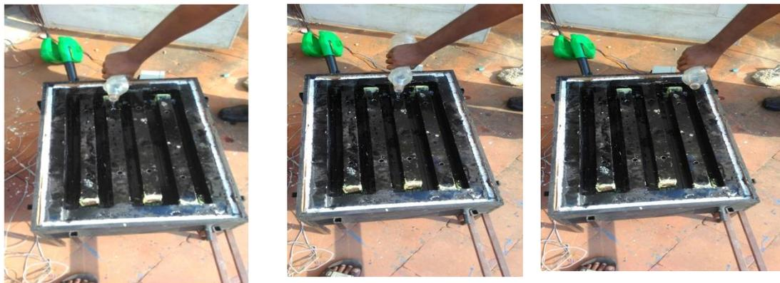
**Figure 4. Assembled view of solar air heater without glass plate**
