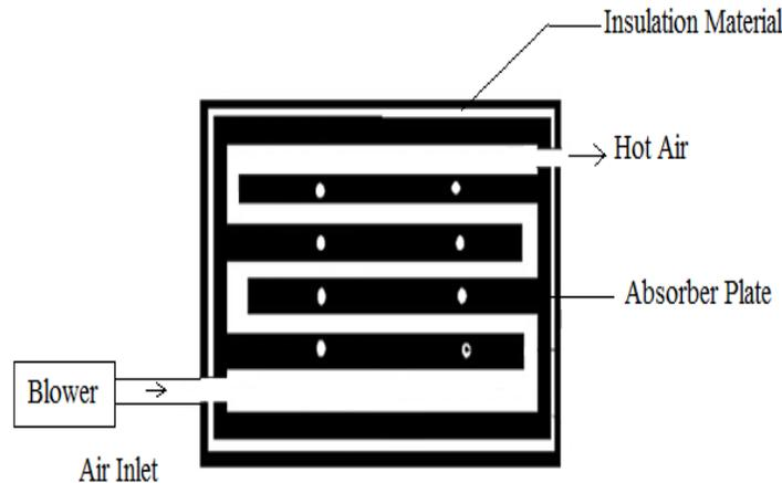
**Figure 2. Schematic Diagram of Solar Air Heater**
