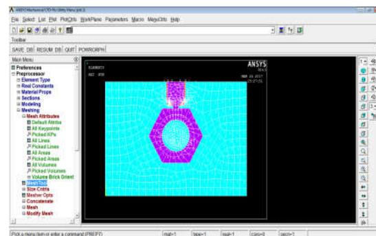
Figure 2. Mesh of the screw Shaped casting
