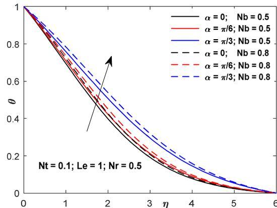
Fig.8: Effects of  $\alpha$  and  $Nb$  temperature profile
