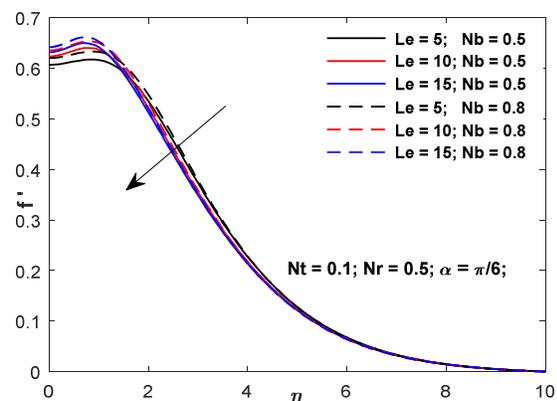
Fig. 4: Effects of  $Le$  and  $Nb$  dimensionless velocity profiles
