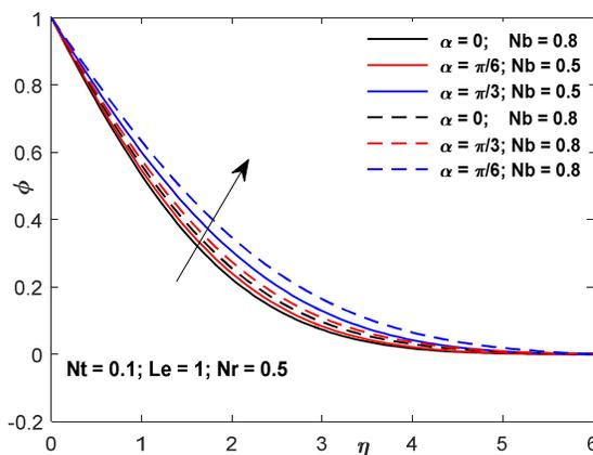
Fig.9: Effects  $\alpha$  and  $Nb$  on the dimensionless Nanoparticle volume fraction profiles
