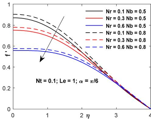
Fig. 1: Effect of  $Nr$  and  $Nb$  on dimensionless velocity.
