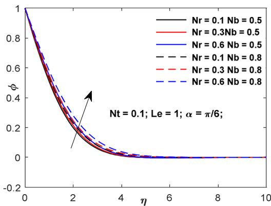
Fig. 3: Effect of  $Nr$  and  $Nb$  on dimensionless nanoparticle volume fraction profiles.
