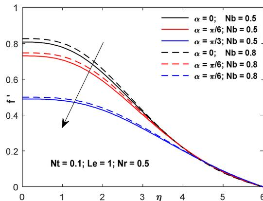
Fig.7: Effects of  $\alpha$  and  $Nb$  on the dimensionless velocity profile
