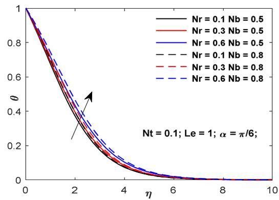
Fig. 2: Effect of  $Nr$  and  $Nb$  on dimensionless temperature profiles
