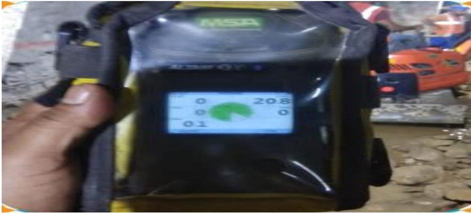
**Figure 5. Hazardous Gas Detector at Different Construction Site**
