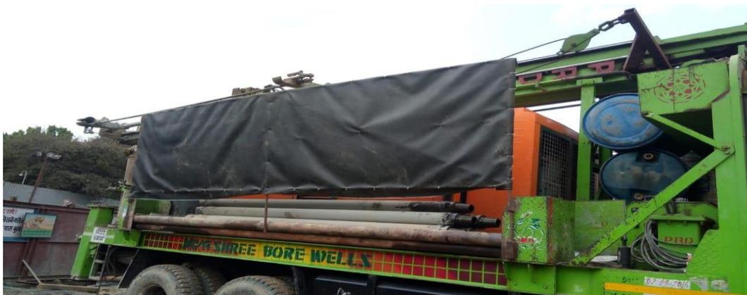
**Figure 3. Noise Barriers around the Compressor of King Post DTH Machine**
