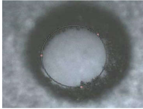
Fig. 4 5.2: Image of micro hole machined in 12th experiment
