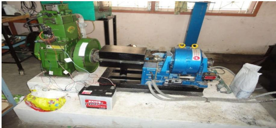
**Figure 3.1: shows pictorial view of engine and dynamometer.**
