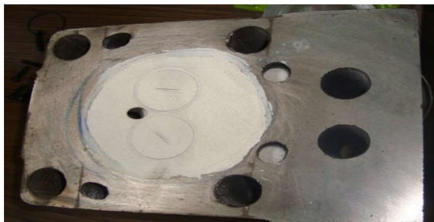
**Figure 3.4: Partially Stabilized Zirconia Coated Cylinder Head**
