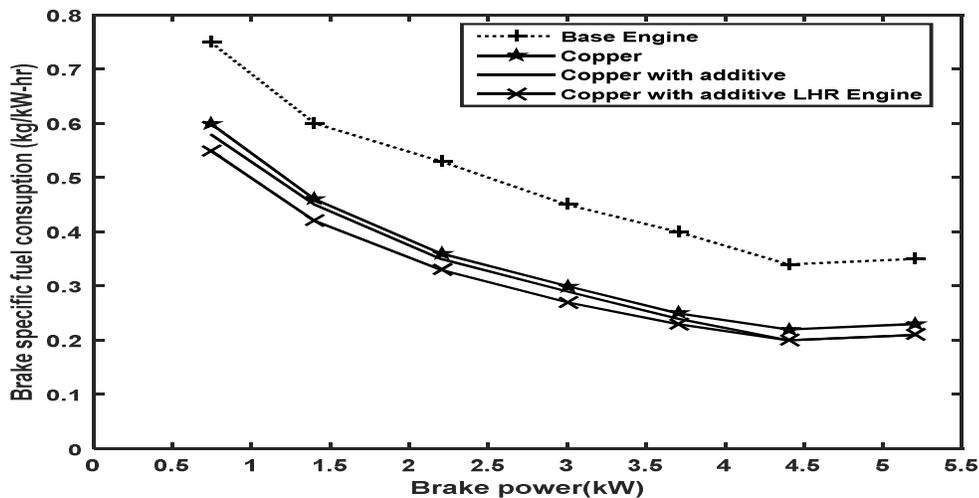
**Figure 4.2: Variation of brake specific fuel consumption with power output for copper piston crown GHI-LHR Engine with Iso-amyle Nitrate additive Ethanol as fuel.**
