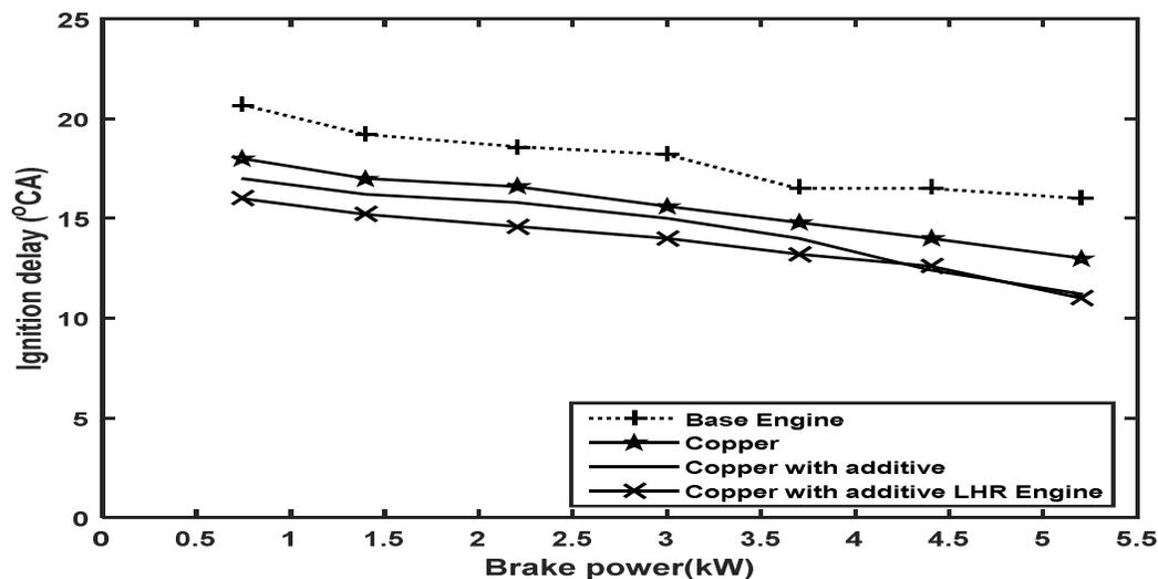
**Figure 4.11: Variation of Ignition delay with power output for copper piston crown GHI-LHR Engine with Iso-amyle Nitrate additive Ethanol as fuel.**
