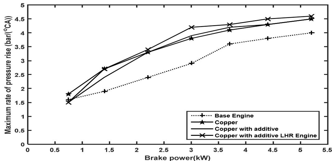
**Figure 4.13: Variation of maximum Rate of Pressure Rise with power output for copper piston crown GHI-LHR Engine with Iso-amyle Nitrate additive Ethanol as fuel.**
