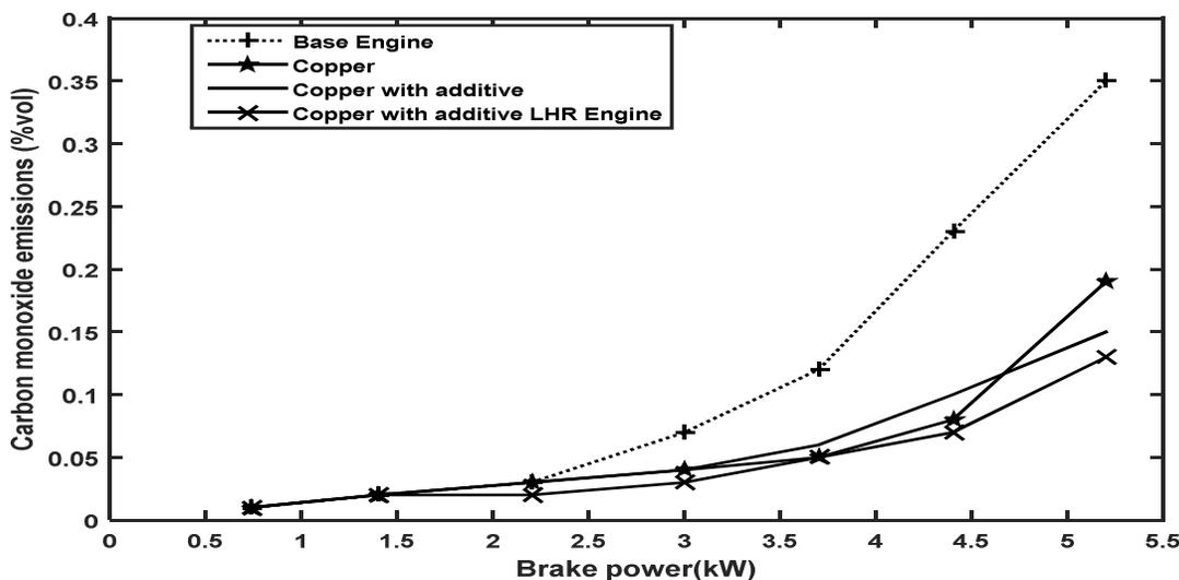
**Figure 4.5: Variation of CO emission with power output for copper piston crown GHI-LHR Engine with Iso-amyle Nitrate additive Ethanol as fuel.**
