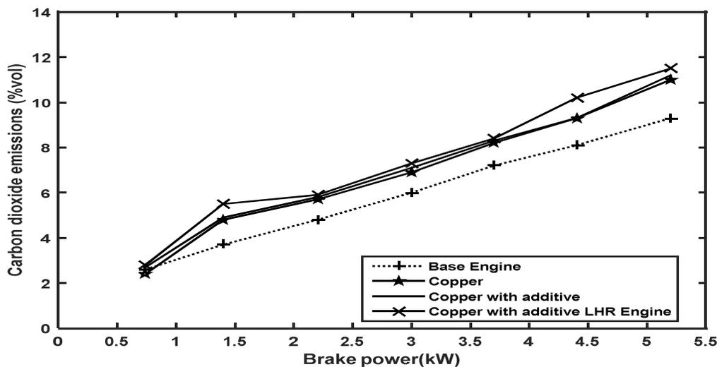
**Figure 4.6: Variation of Carbon dioxide with power output for copper piston crown GHI-LHR Engine with Iso-amyle Nitrate additive Ethanol as fuel.**
