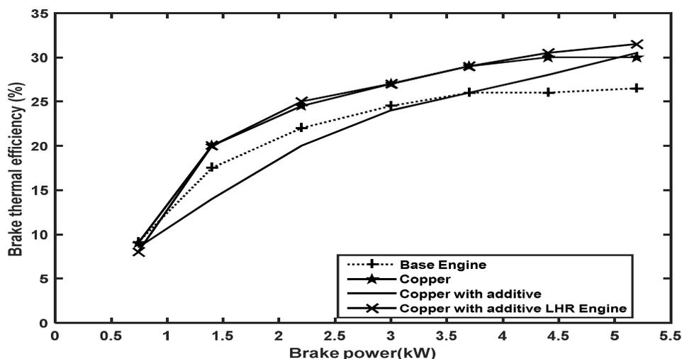
**Figure 4.1: Variation of Brake thermal efficiency with power output for copper piston crown GHI-LHR Engine with Iso-amyle Nitrate additive Ethanol as fuel.**
