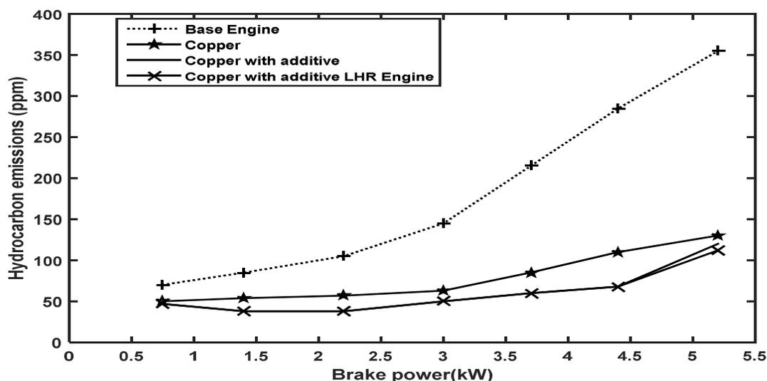
**Figure 4.4: Variation of Hydrocarbons with power output output for copper piston crown GHI-LHR Engine with Iso-amyle Nitrate additive Ethanol as fuel.**
