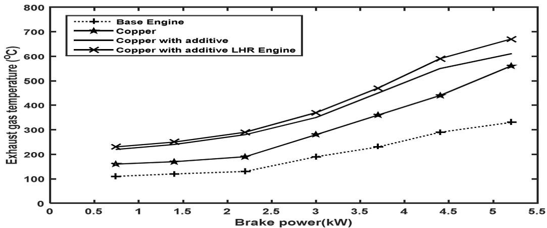
Figure 4.9: Variation of Exhaust gas temperature with power output for copper piston crown GHI-LHR Engine with Iso-amyle Nitrate additive Ethanol as fuel.
