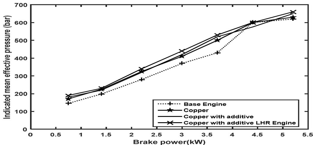
**Figure 4.12: Variation of Indicated mean effective pressure with power output for copper piston crown GHI-LHR Engine with Iso-amyle Nitrate additive Ethanol as fuel.**
