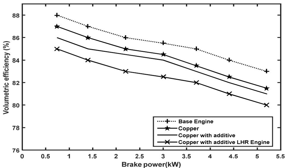
**Figure 4.3: Variation of Volumetric efficiency with power output for copper piston crown GHI-LHR Engine with Iso-amyle Nitrate additive Ethanol as fuel.**
