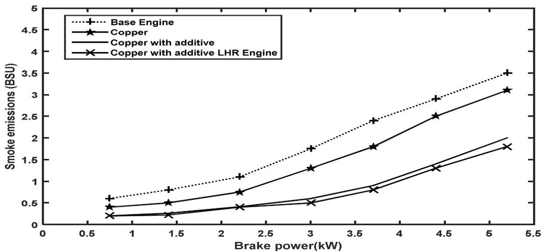
**Figure 4.8: Variation of Smoke Emission with power output for copper piston crown GHI-LHR Engine with Iso-amyle Nitrate additive Ethanol as fuel.**
