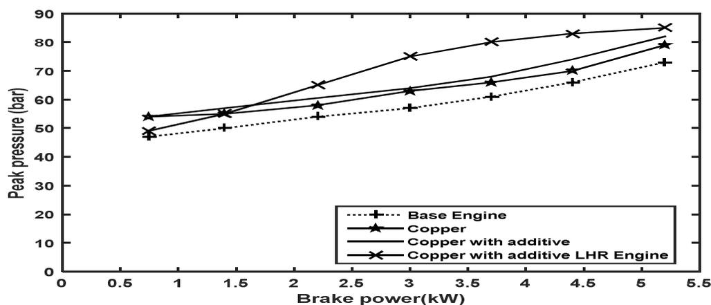
Figure 4.10: Variation of Peak Pressure with power output for copper piston crown GHI-LHR Engine with Iso-amyle Nitrate additive Ethanol as fuel.
