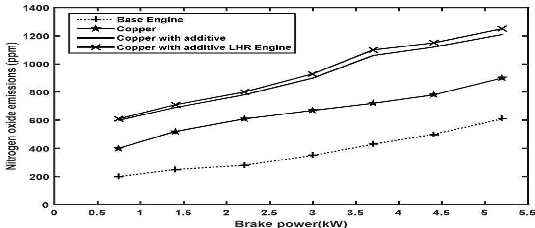
**Figure 4.7: Variation of NOx emission with power output for copper piston crown GHI-LHR Engine with Iso-amyle Nitrate additive Ethanol as fuel.**
