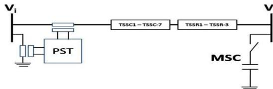
Fig.1 Per phase schematic diagram of HFC
