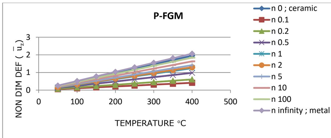
**Figure 1: Effect of variable thermal environment on non-dimensional deflection ( $\bar{u}_z$ ) for simply supported square plate (P-FGM)**
