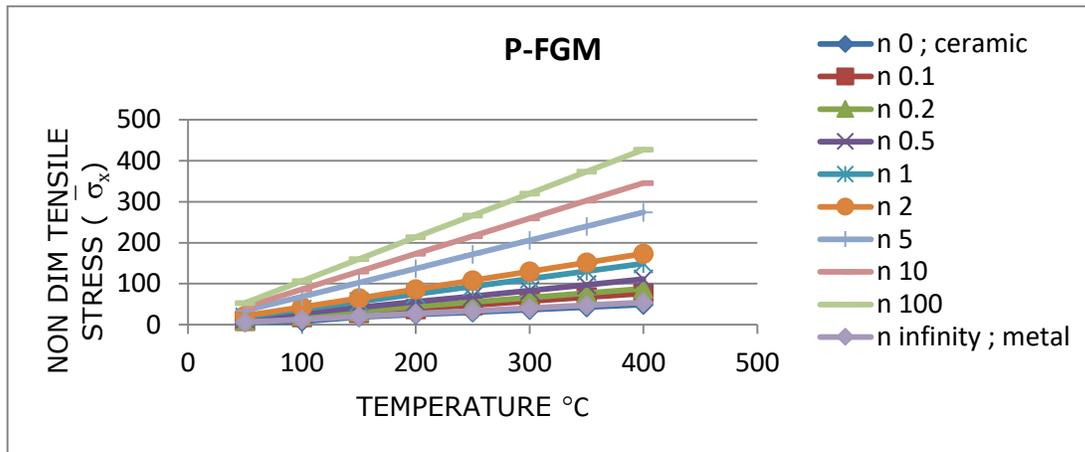
**Figure 3: Effect of variable thermal environment on non-dimensional tensile stress ( $\bar{\sigma}_x$ ) for simply supported square plate (P-FGM)**
