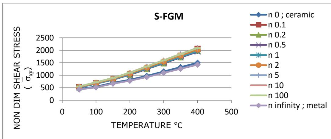
**Figure 12: Effect of variable thermal environment on non-dimensional shear stress ( $\overline{\sigma_{xy}}$ ) for simply supported plate under constant mechanical load for S-FGM**
