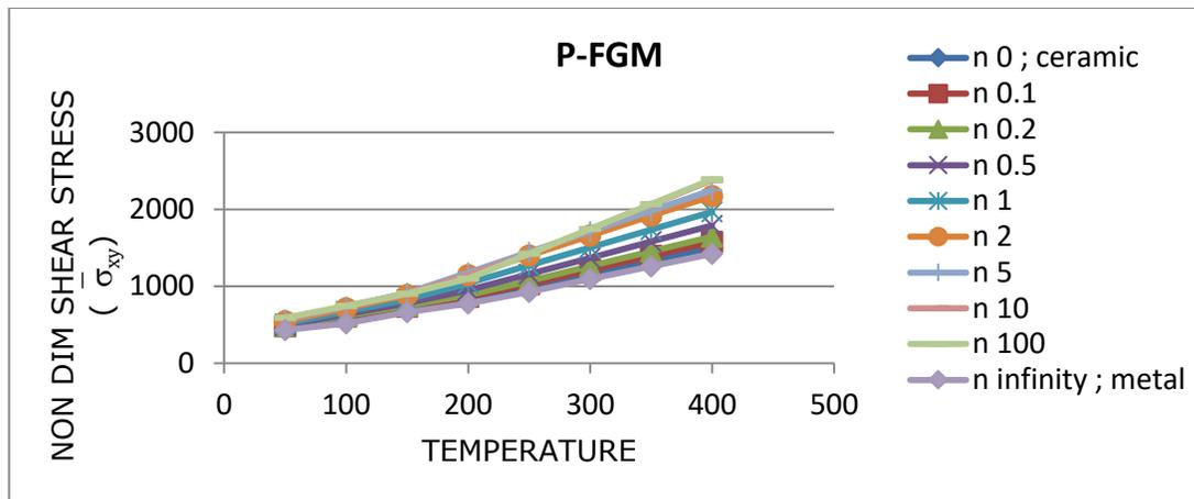
**Figure 11: Effect of variable thermal environment on non-dimensional shear stress ( $\overline{\sigma_{xy}}$ ) for simply supported plate under constant mechanical load for P-FGM**
