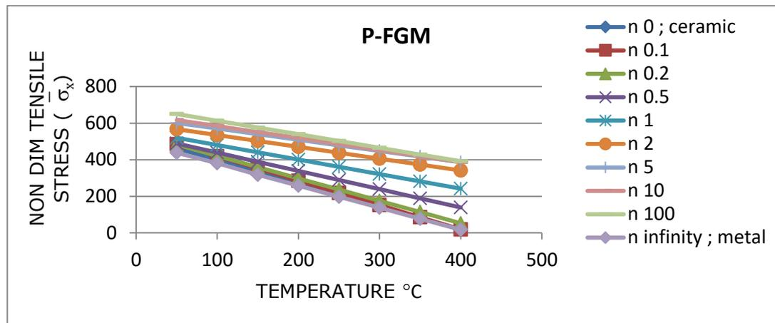
**Figure 9: Effect of variable thermal environment on non-dimensional tensile stress ( $\bar{\sigma}_x$ ) for simply supported plate under constant mechanical load for P-FGM**
