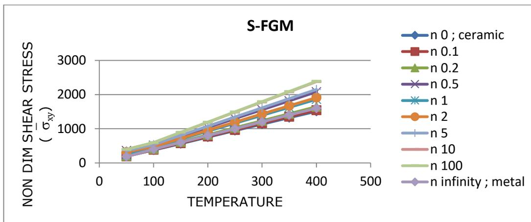
**Figure 6: Effect of variable thermal environment on non-dimensional shear stress ( $\overline{\sigma_{xy}}$ ) for simply supported square plate (S-FGM)**
