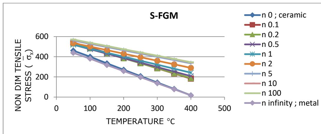
**Figure 10: Effect of variable thermal environment on non-dimensional tensile stress ( $\bar{\sigma}_x$ ) for simply supported plate under constant mechanical load for S-FGM**
