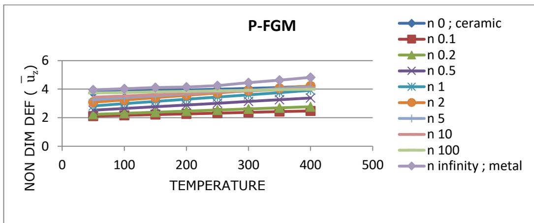
**Figure 7: Effect of variable thermal environment on non-dimensional deflection ( $\bar{u}_z$ ) for simply supported plate under constant mechanical load for P-FGM**
