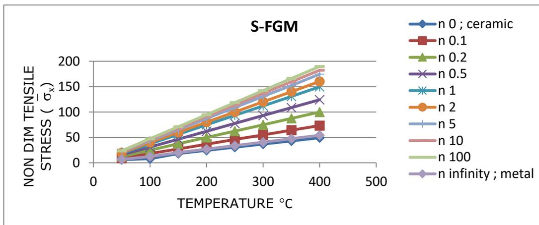
**Figure 4: Effect of variable thermal environment on non-dimensional tensile stress ( $\bar{\sigma}_x$ ) for simply supported square plate (S-FGM)**
