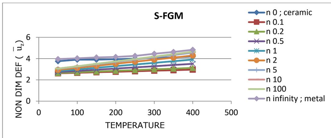
**Figure 8: Effect of variable thermal environment on non-dimensional deflection ( $\bar{u}_z$ ) for simply supported plate under constant mechanical load for S-FGM**
