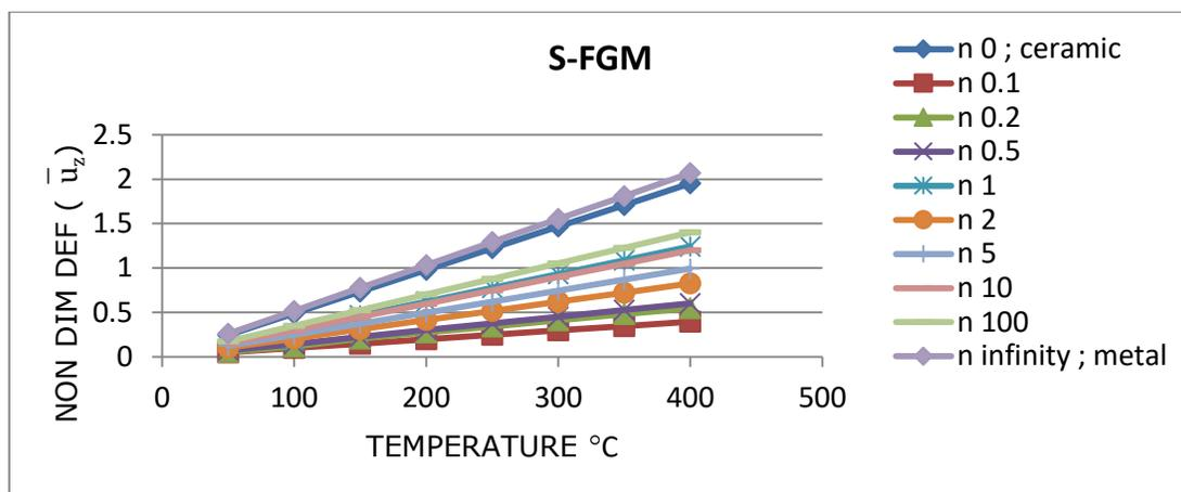
**Figure 2: Effect of variable thermal environment on non-dimensional deflection ( $\bar{u}_z$ ) for simply supported square plate (S-FGM)**
