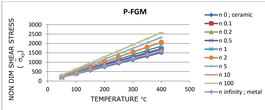
**Figure 5: Effect of variable thermal environment on non-dimensional shear stress ( $\overline{\sigma_{xy}}$ ) for simply supported square plate (P-FGM)**
