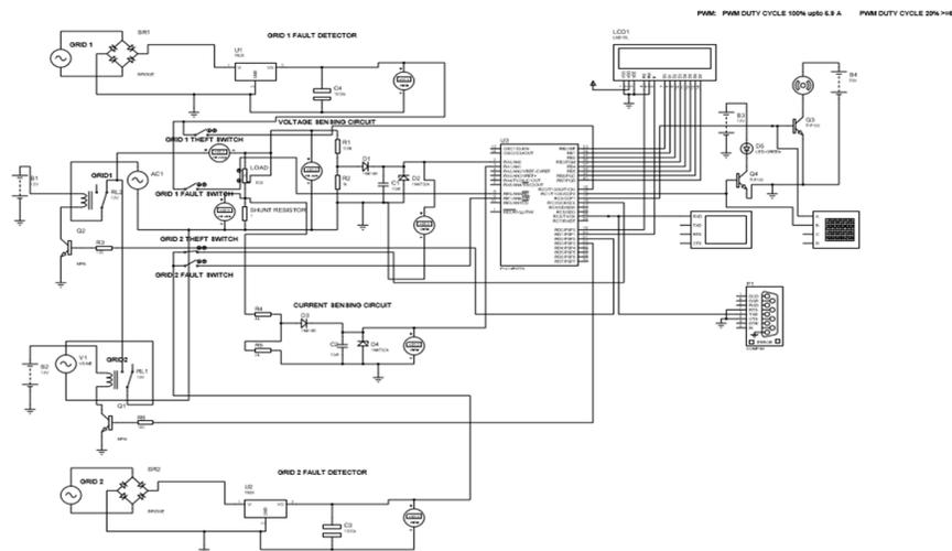
FIGURE 4:- SIMULATION CIRCUIT DIAGRAM OF IOT BASED SMART GRID IN ISIS PROFESSIONAL
