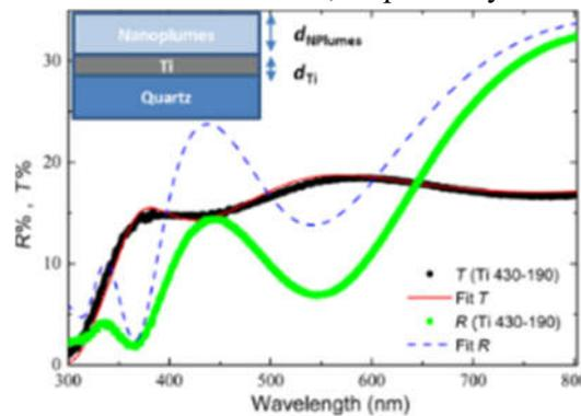
**Figure 1: Fitting of the transmittance and reflectance spectra of Ti (430-190).**
