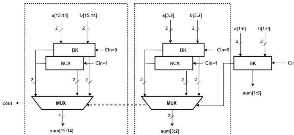
Figure 4.Schematic diagram for Carry Select Adder using Brent Kung adder
