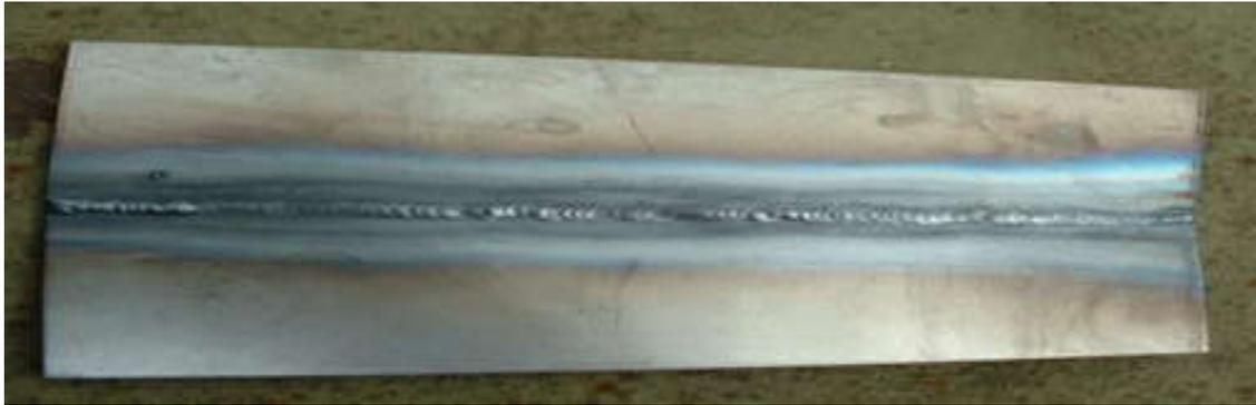
**Figure 4. TIG Welded Sample**
