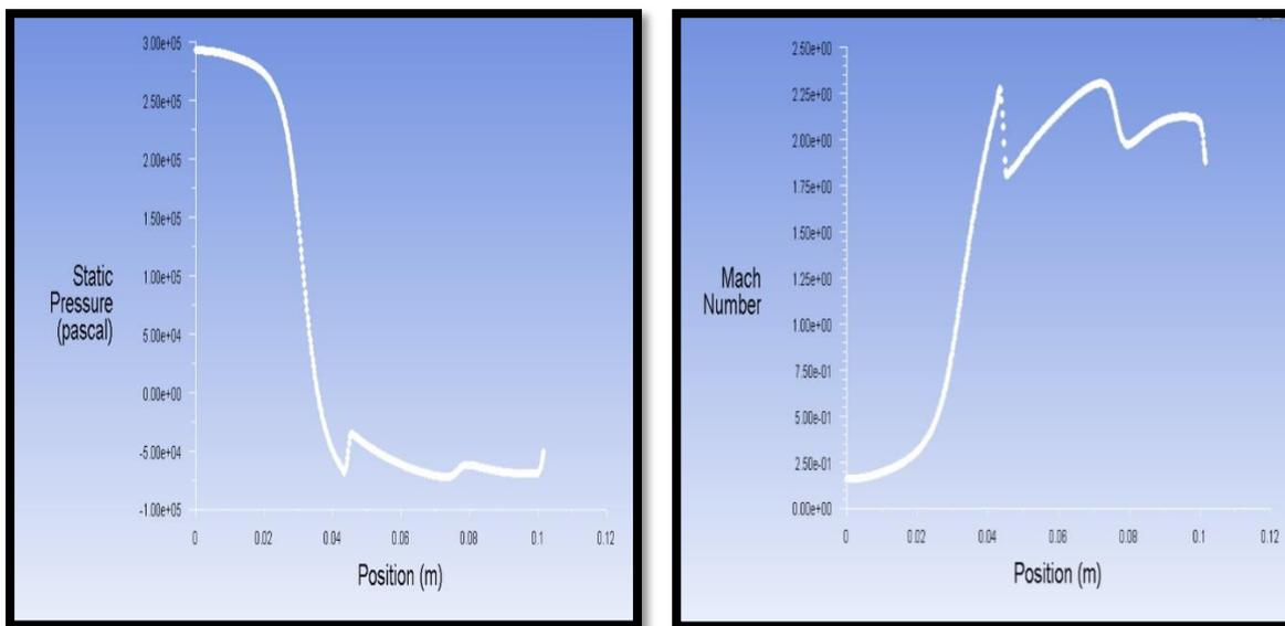
Figure 5: Graph of standard turbulent model for the (a) static pressure vs position (m) and (b) mach number vs position (m)
