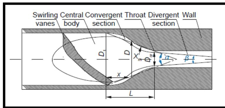
Fig 1: Structure of the nozzle [1]
