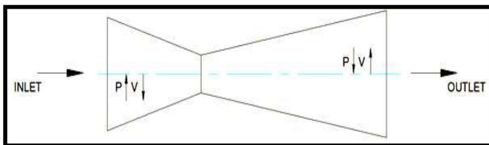
Fig 2: Principle of C-D Nozzle [2]
