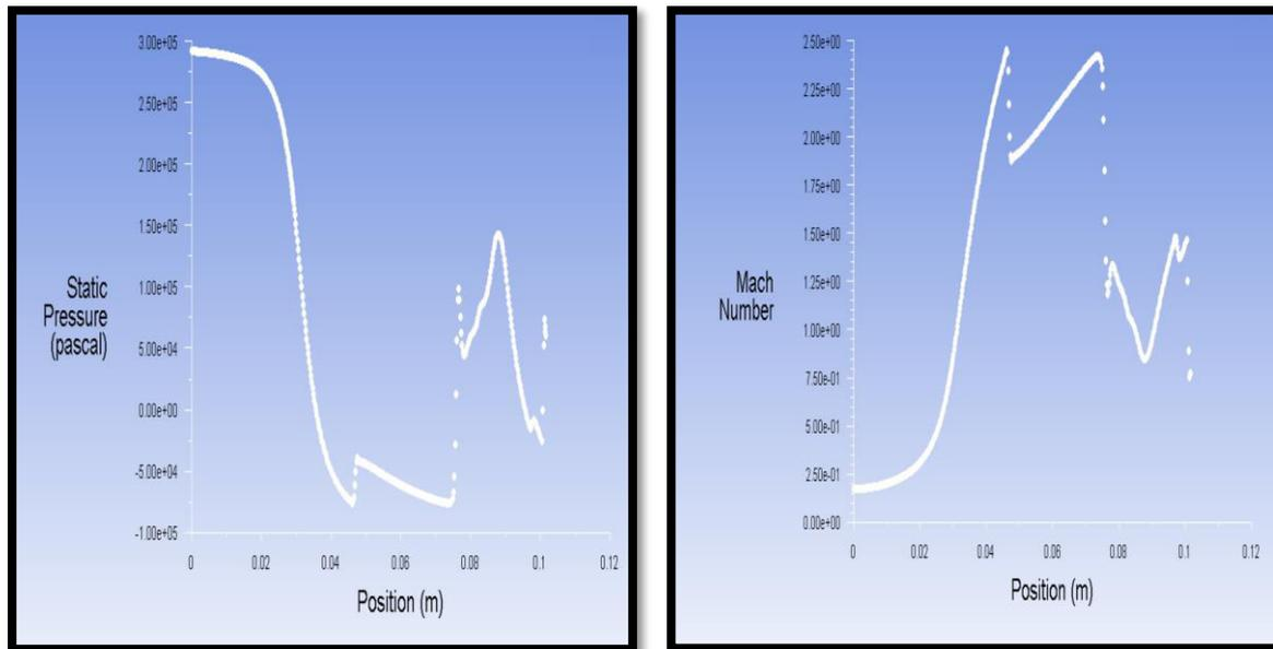
Figure 6: Graph of realizable turbulent model for the (a) static pressure vs position (m) and (b) mach number vs position (m)
