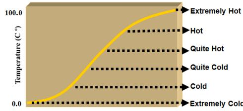
Figure 4. Fuzzy Logic (for ‘Temperature’)
