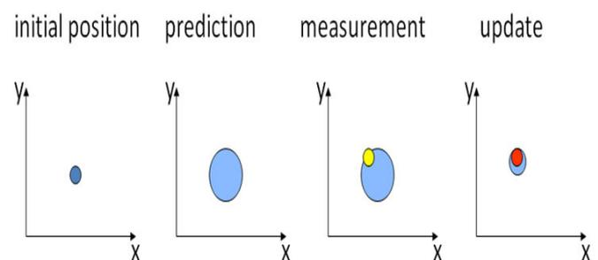
Fig. 1. Schematic views of Kalman filter tracking idea.
