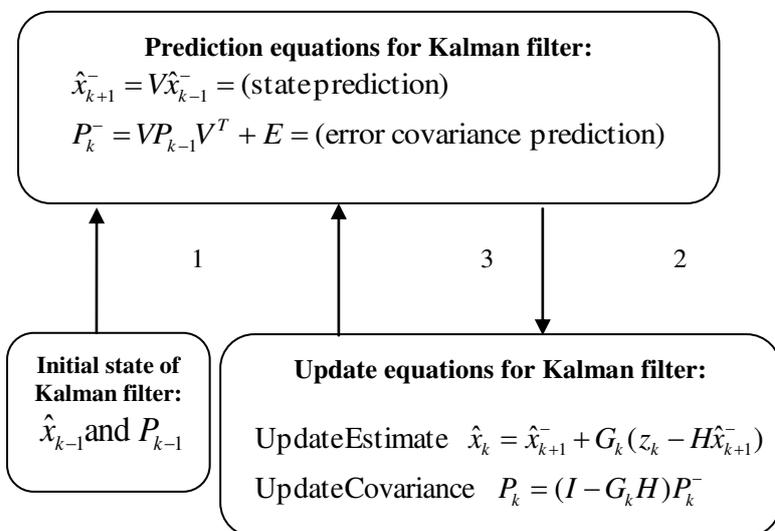
Above flow charts shows the Kalman Filter (KF) algorithm Iteration. Where ‘1’ shows initial state equation of the algorithm after that ‘2’ shows the prediction equations and finally ‘3’ shows the updating in the prediction equation which helps to predict the future position of the object.
